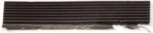
**Prevention:** Check alignment periodically as detailed above. Grease the idler arm once a week during spraying season and prior to winter storage.
